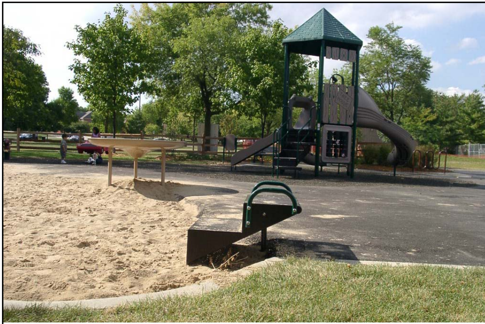
Sand area with transfer system for lowering into sand and adjacent elevated sand table.
