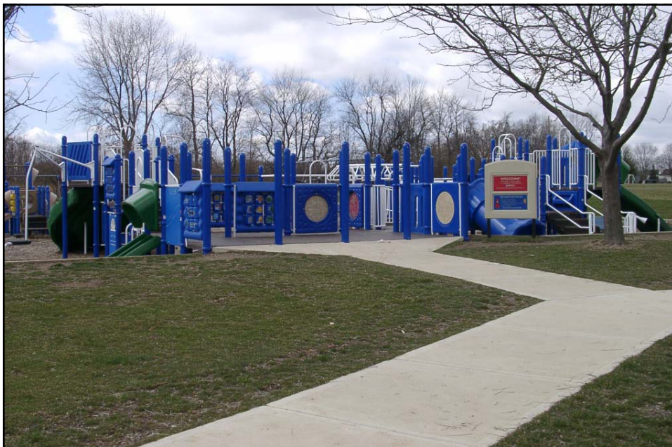
A landscaped berm access route, less than 1:20 with a concrete path, leads to the upper deck of a large composite play structure.
